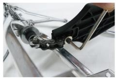
Use the wrench supplied with CHS-1 to remove the chain screw.
